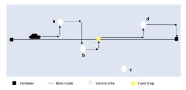
Example of an FRT line, with two terminals, an intermediate fixed stop (in yellow) and the service area in grey, along with a tentative route for the shuttle allowing to serve the demands a, b and d while also serving the fixed stops.
